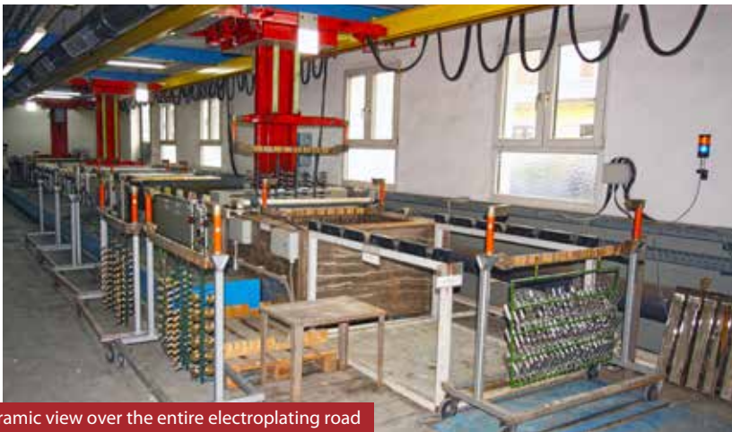
Framed components chrome-plated, in production
